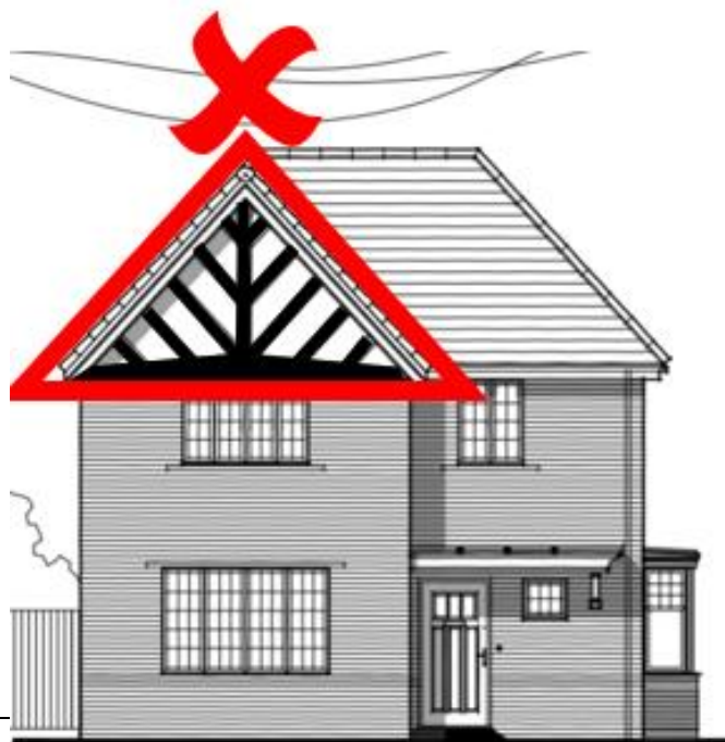
figure 9: Removal of mock 'Tudorbethan' style framing in gables
